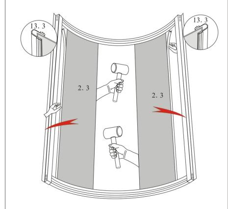
Installing fixed glass take off aluminum alloy water bar then install water dar after installingfised glass and aluminum panel
